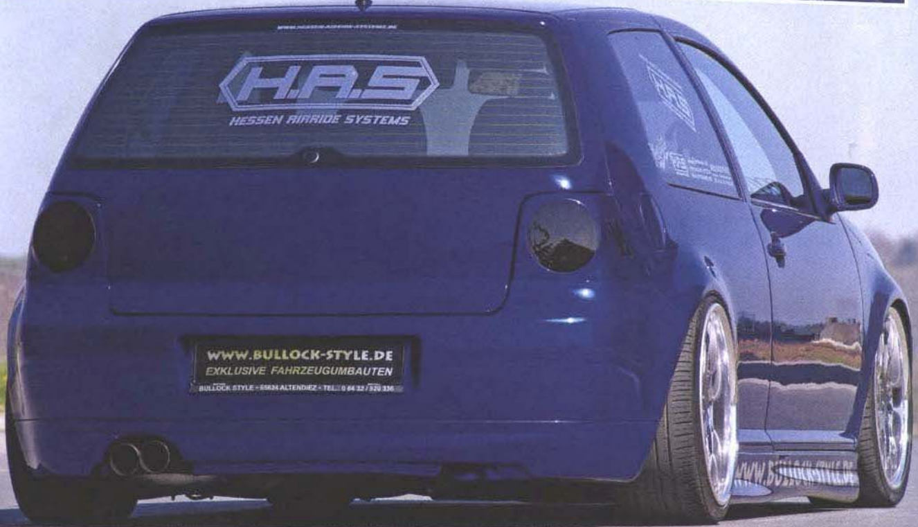
(left) Painted light housings leave tail light and separate indicators exposed. Four triangles in round light act as brake, indicator, reverse, etc
